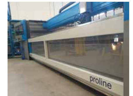
Front and rear hatch with pneumatic movement to better protect the cutting area and reduce the dispersion of water and abrasive material
