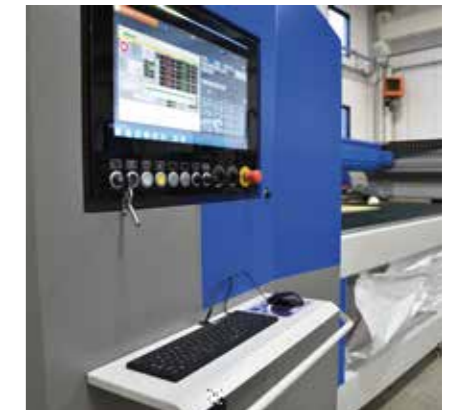
21.5" industrial PC Panel on the machine with touch display and HMI CMS Active interface
